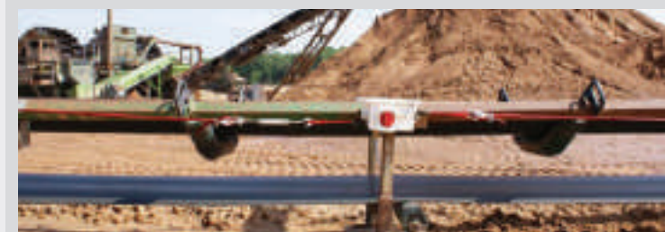
Pullswitch installed on open belt conveyor
