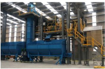
Our client developed a greenfield store for the storage and dispatch of fertiliser to its shareholders. We fabricated, installed, and commissioned blending hoppers, a bucket elevator screen, lump breaker, belt conveyors, structural steel, and chutes.
